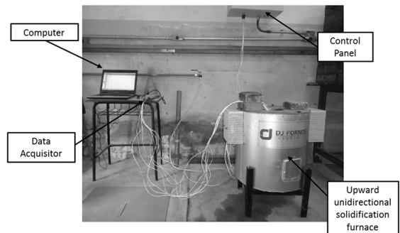
Figure 2. Upward unidirectional solidification furnace with control panel, data acquisition unit connected to thermocouples and computer to present and store experimental data.
