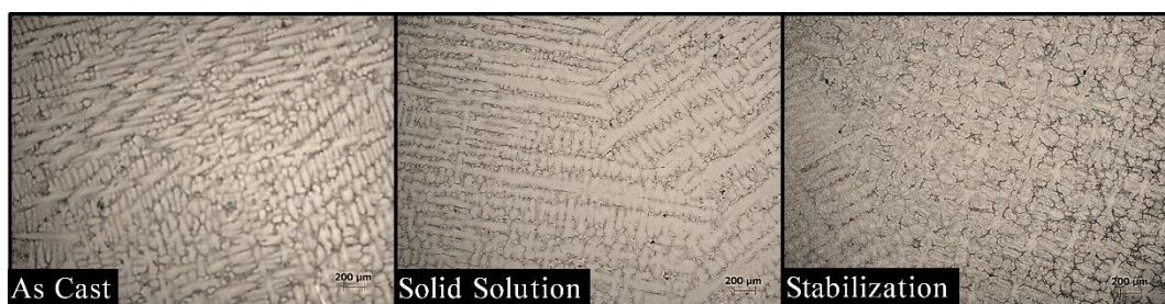
Figure 3. Images obtained by optical microscopy of the Inconel 713C material as cast, solid solution heat treated and stabilization heat treated condition.
