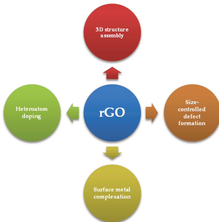
Figure 1. General schematic roadmap of defect engineering strategies in reduced graphene oxide support materials for achieving advanced energy conversion.
