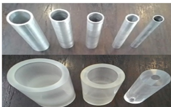
Fig. 1. Cylindrical absorber layer made of aluminum and PMMA built to form the Tandem system.
