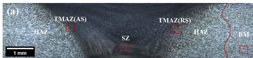
Fig. 2. Cross section of the friction stir welded joint. The dashed red boxes indicate the regions where EBSD maps were acquired. (For interpretation of the references to colour in this figure legend, the reader is referred to the Web version of this article.)
