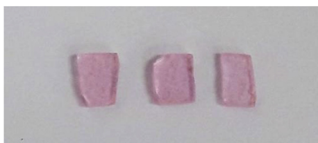
Fig. 1. Aliquots of 3 mol% Er-doped phosphate glass used in this study.
