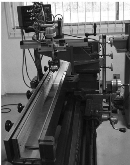
Fig. 6. Details of the side plates positioning in the roll swaging bed.
