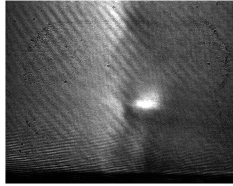
Fig. 8. Superposition of the Schlieren and plasma images, showing where typically the plasma forms. The laser pulses came from the right.
