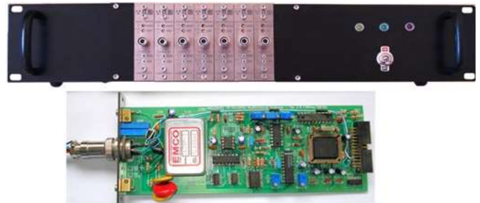
Figure 3 -- The multichannel module (top) and one of seven eight bit resolution multichannel board (bottom).
