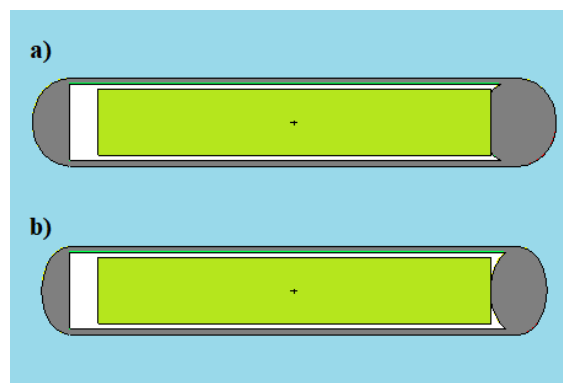
Figure 3: Two seeds modeled with different end-weld thickness a) 4.50 mm length seed; b) 4.67 mm length seed
