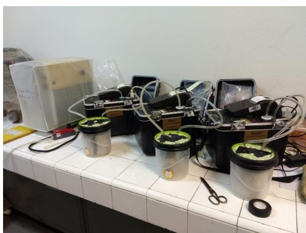
Figure 4: Experimental arrangement for radon exhalation rate measurement in proof bodies samples.
