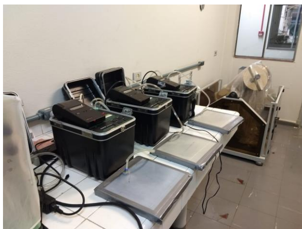
Figure 3: Experimental arrangement for radon exhalation rate measurement in plate samples.
