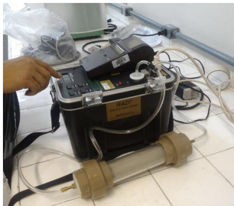
Figure 2: Experimental arrangement for radon exhalation rate measurement in aggregate samples.
