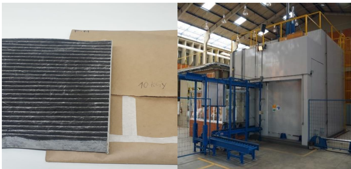
Figure 4: Sample package and multipurpose irradiator, IPEN/CTR.
