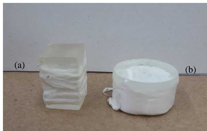
Figure 1- Grown crystals of CsI(Tl) size (a) \square 12.3 x \downarrow 19.5 (parallel face and thickness) and (b) cylinder with dimensions of \varnothing 20.1 x \uparrow 11.9 (circular face and thickness). All dimensions are in millimeters.
