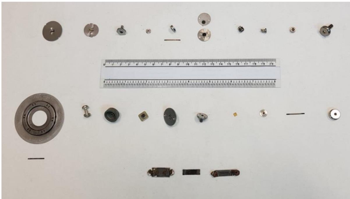
Figure 1: Types of Am-241 sources of smoke detectors (rows 1 and 2) and lightning rods (row 3)
