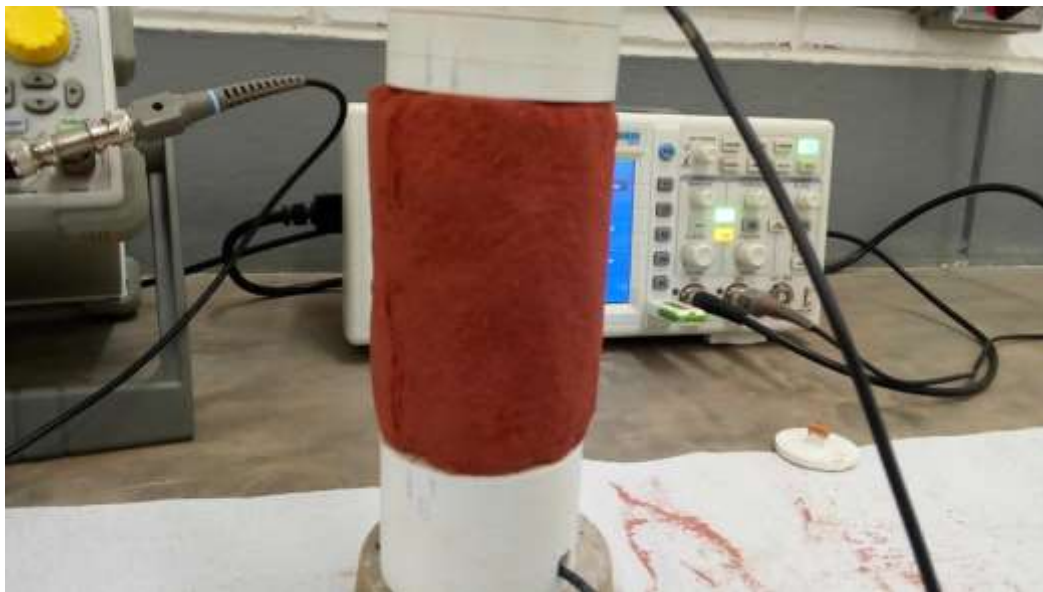
Figure 3: Probe used in the bender elements test
