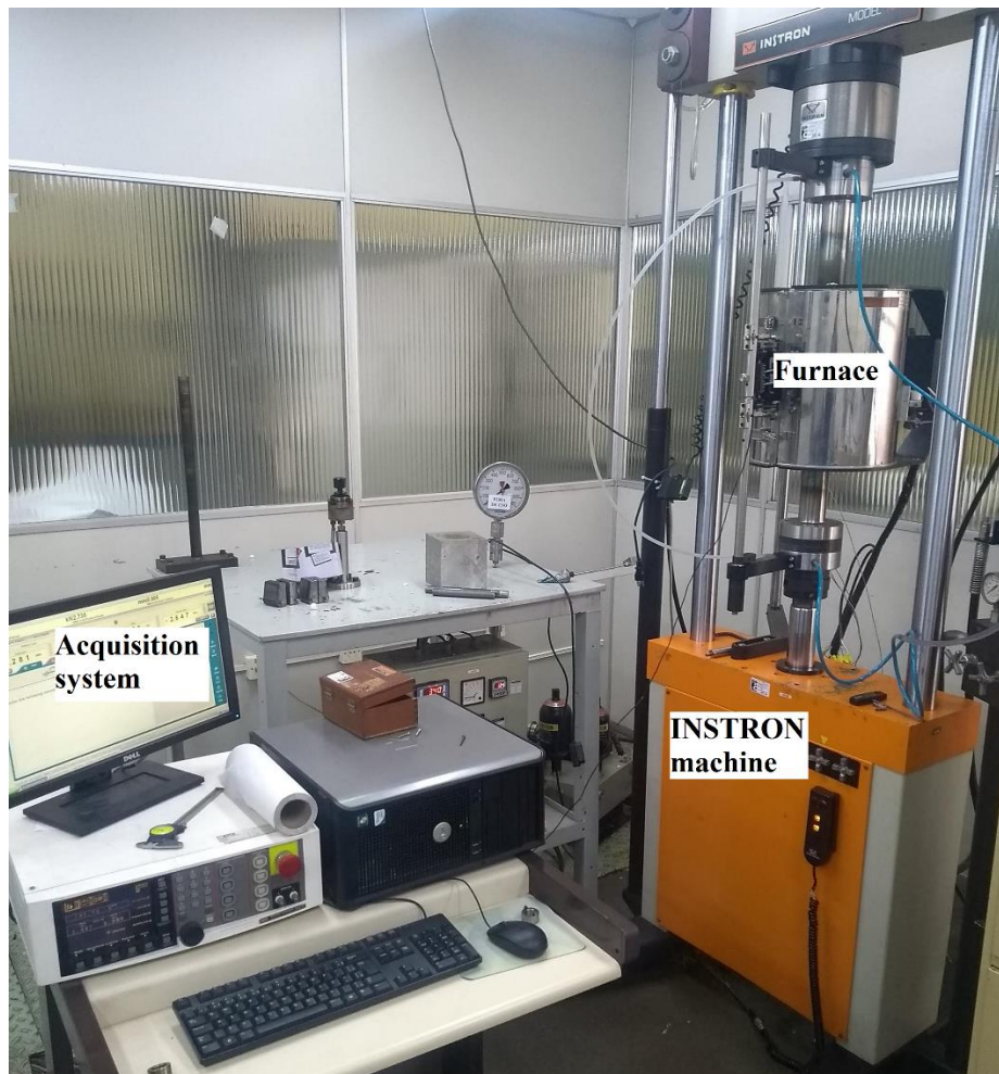
Figure 3 - Experimental apparatus for tensile test on the INSTRON Testing Machine.
