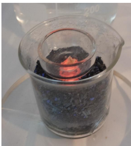
Figure 1: View of the test apparatus, showing the hot spot in the sample-holder.
