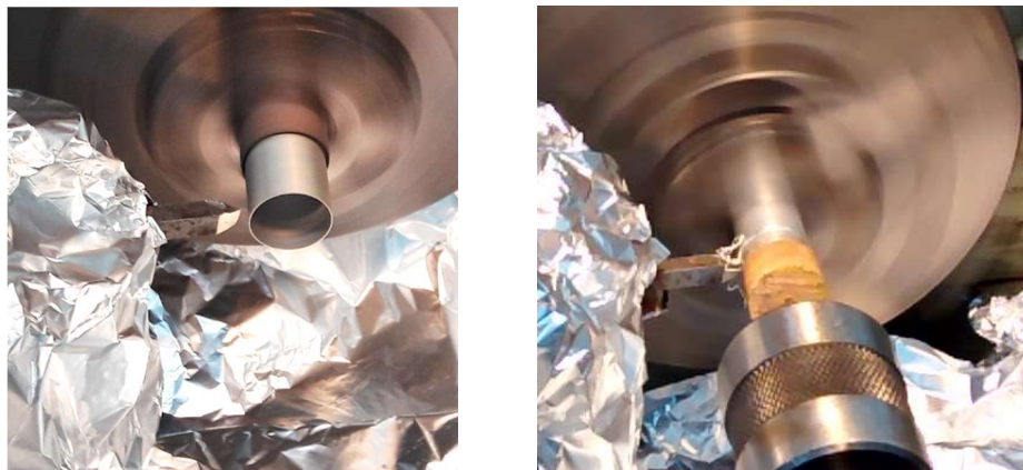
Figure 8: Cutting tool test, tool aspect (left), making a cut (right).
