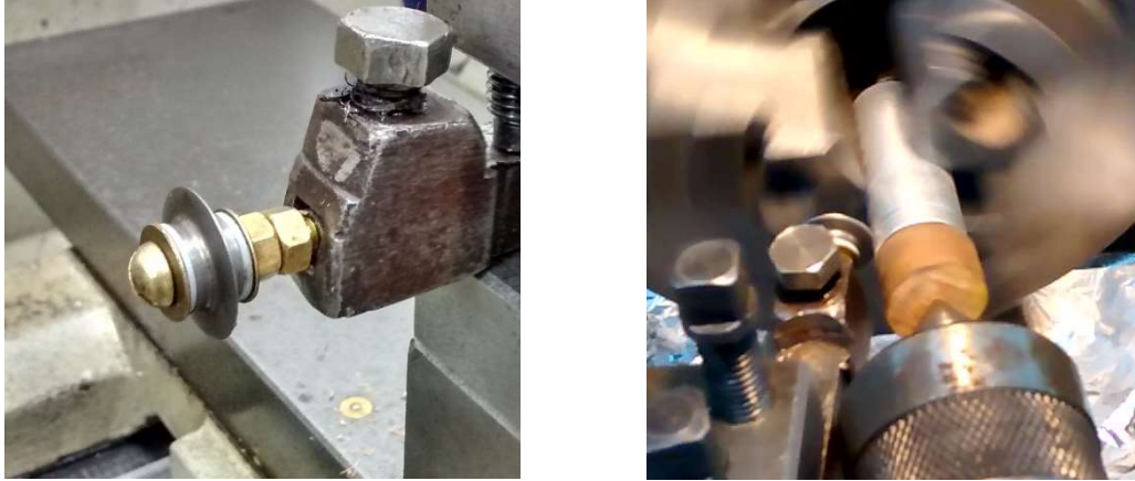
Figure 9: Wheel blade test, tool aspect (left), making an opening (right).
