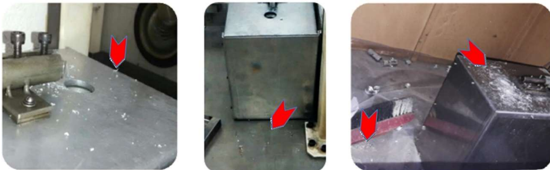
Figure 4: Radioactive aluminum debris around the opening device after a cut performed.
