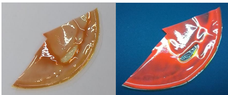
Figure 1: PMMA:Ag:Eu(tta) 3 (TPPO) 2 film without and with the presence of UV radiation.
