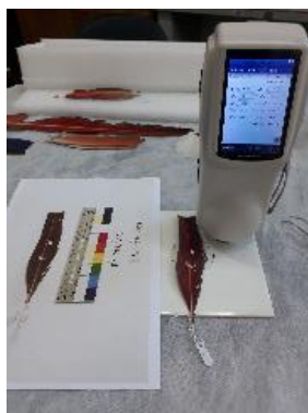
Figure 4: Colorimeter and feather measurement setup.
