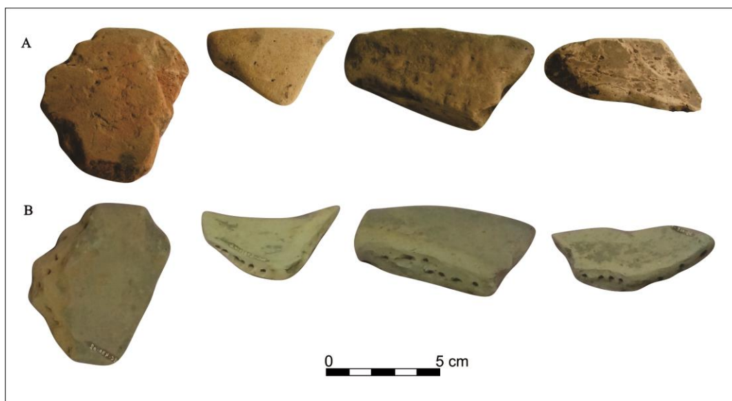
Figure 6: Samples before preparation (A); Samples after preparation with holes on the side of the part (B).
