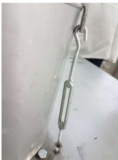
Figure 4: In particular, cable tensioner used to secure the barrel.
