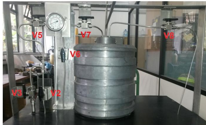
Figure 6: AISI 304 stainless steel tubing with 6.35 mm (1/4") inner diameter (superior level) and needle valves (V2-V8) [9].
