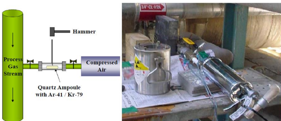
Figure 2: Injection of the gaseous radioisotopes ( ^{41}\text{Ar} or ^{79}\text{Kr} ) in tubes and vessels submitted to low or medium pressures [6].
