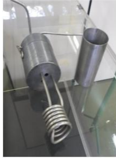
Figure 9: Liquid nitrogen based freezing system for gas liquefaction [9].
