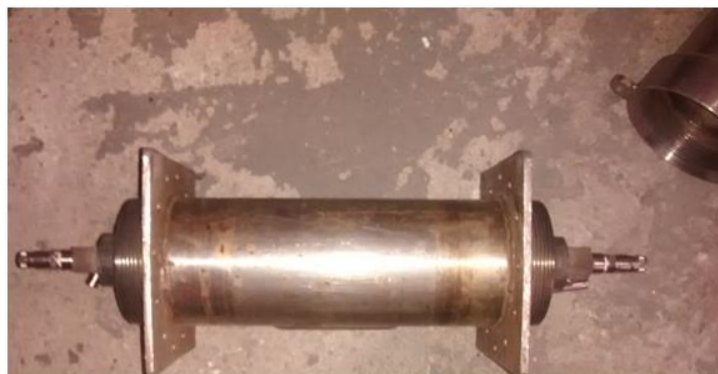
Figure 12: Cylinder for storage and transportation of the gaseous radiotracers [9].
