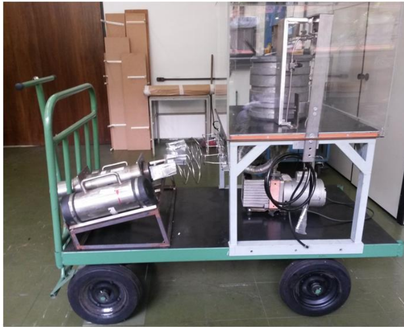
Figure 4: Irradiation system for production of gaseous radioisotopes [9].
