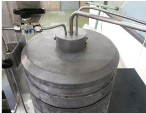
Figure 10: Lead shielding for the liquefaction dewar [9].
