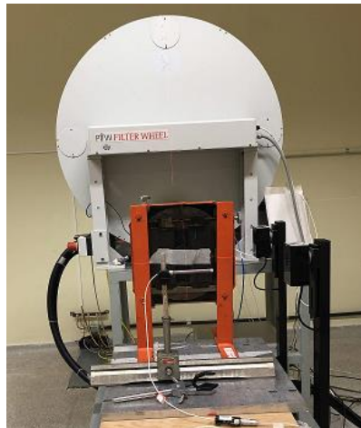
Figure 2. Schematic assembled for obtain Kerma rate values.
