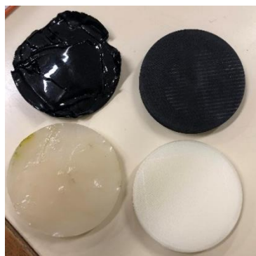
Figure 3. Samples printed in transparent PLA and black ABS for comparison with recycled samples
