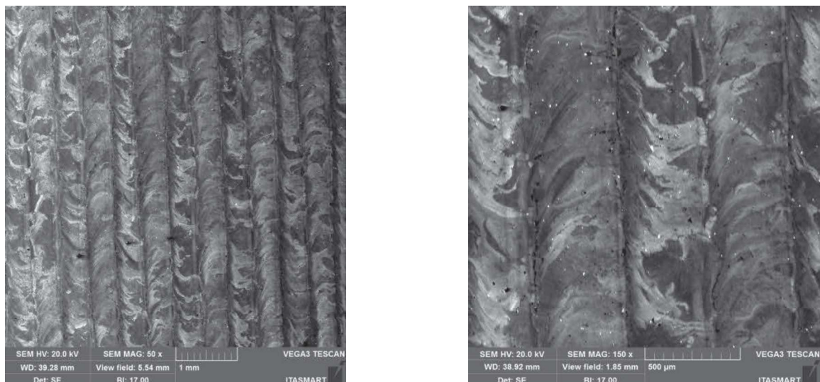
Fig. 1. Micrograph maraging 300 steel surface treated with magnification of (a) 50x and (b) 150x.
