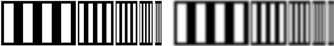
Figure 3: A series of bars in different resolutions is used to compute MTF (modular transfer function).
