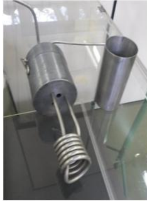
Figure 6. Liquid nitrogen based freezing system for gas liquefaction.
