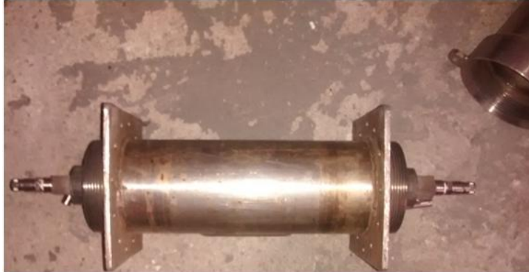
Figure 9. Cylinder for storage and transport of the gaseous radiotracers.
