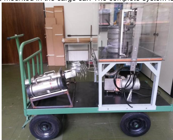
Figure 12 – System to load and unload the irradiation capsule placed inside the IEA-R1's water pool.
