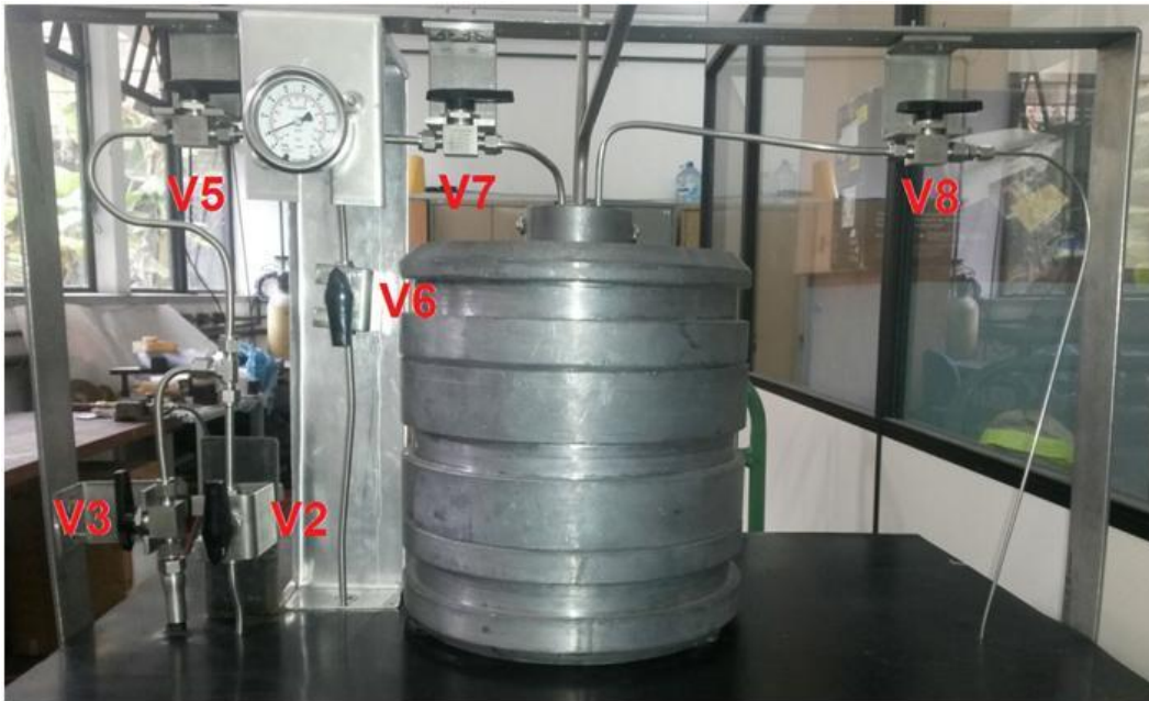
Figure 3. AISI 304 stainless steel tubing with 6.35mm (1/4") inner diameter (superior level) and needle valves (V2-V8).
