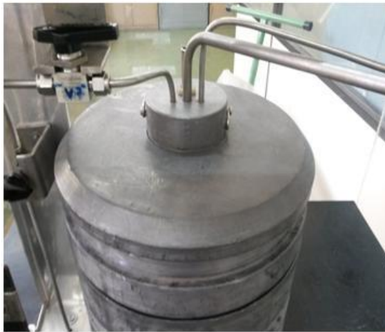
Figure 7. Lead shielding for the liquefaction dewar.
