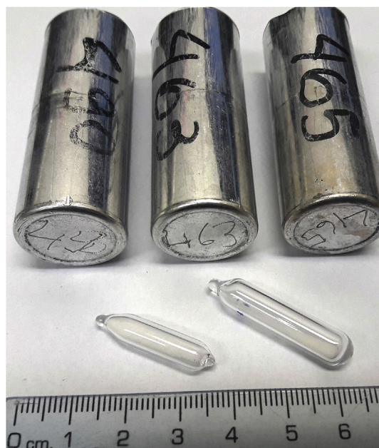
Fig. 1. Silica and aluminum tubes used during the irradiation of the \text{CaSiO}_3 samples in the IEA-R1 reactor.
