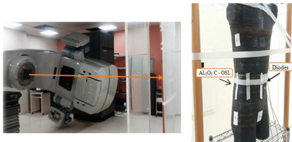
Fig. 4. a) TSEB experimental set-up of irradiation using the AldersonRando® anthropomorphic phantom. Distance between the phantom and the field isocenter is 3 m and (b) location of Al_2O_3:C dosimeters and Silicon DIODES.
