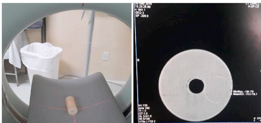
Fig. 4. Tests with the samples in a computed tomography equipment to obtain the equivalence of the materials to human tissues by CT number.
