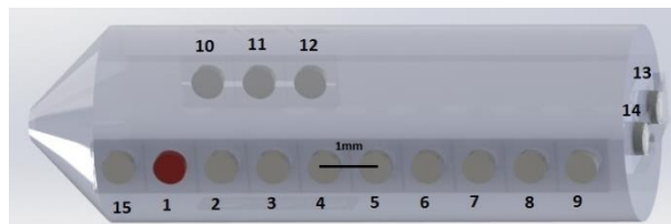
Figure 1: Thermoluminescent dosimeters along the conical tube. The red region (dosimeter 1) refers to the location of the mouse breast. The distance between the dosimeter 1 and 10 (posterior to the breast) is around 3 cm. The dosimeters 13 and 14 represent the head region and the dosimeter 15 represents the tail region of the mouse.
