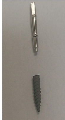
Figure 1 – Dental implant of Ti grade V and a prosthetic abutment of stainless steel 316L.
