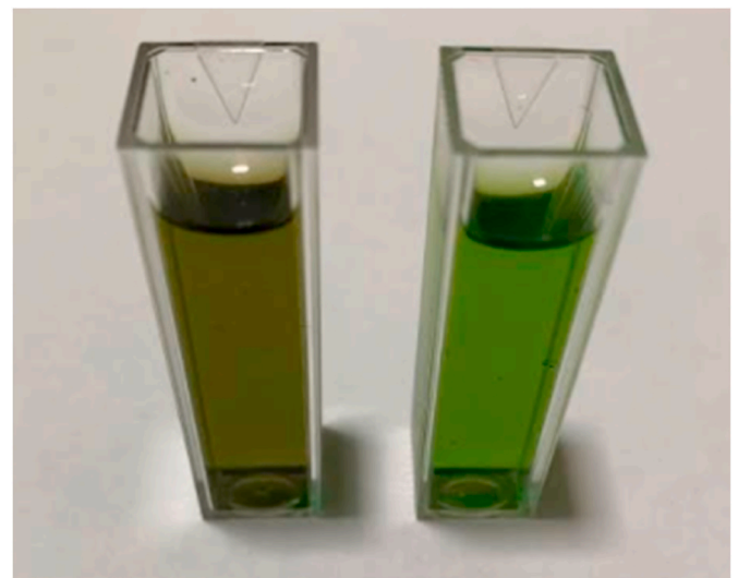
Fig. 3. FXL-mblue samples: on the left side non-irradiated sample (0.00 kJ/cm 2 ) and on the right side irradiated sample (21.6 kJ/cm 2 ).
