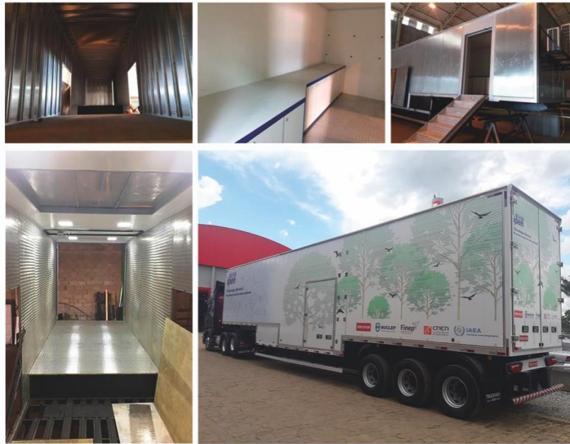
Figure 4. Construction of the IPEN-CNEN/SP's mobile electron beam irradiation unit.
