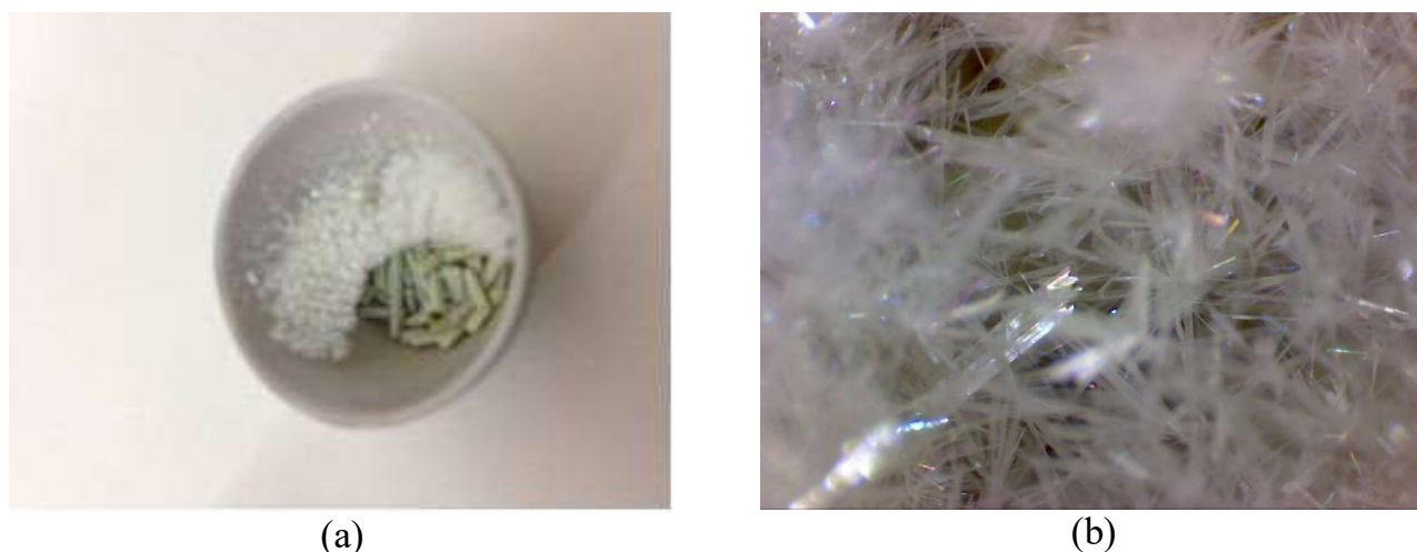
Fig. 8. Radiation-thermal treatment (RTT) processing on spent Hydro Catalytic Cracking (HCC) catalyst from upper zone: a) alumina crucible and b) crystal formed after electron beam irradiation.
