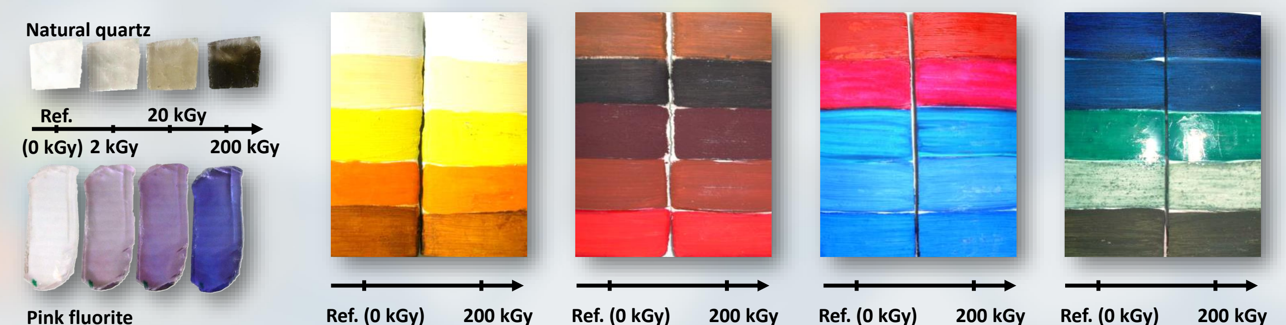
While transparent materials like gemstone tint easily under photon or electron irradiation, opaque materials, such as polychrome layers (here different classic pigments in poppy seed oil on gesso coated wooden samples), do not.
