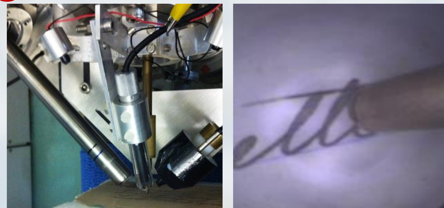
External ion beam set-up at C2TN. 2 MeV proton beam is used to measure iron gall ink in an ancient manuscript.
