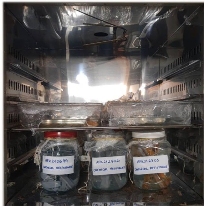
Fig. 1. Oven with controlled temperature for specimens storage.
