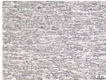
Figure 1. Typical microstructure of 22MnB5 steel in as-received state.
