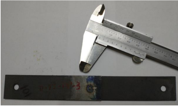
Figure 6: Detail of a specimen for tension shear tests, ready to be tested.
