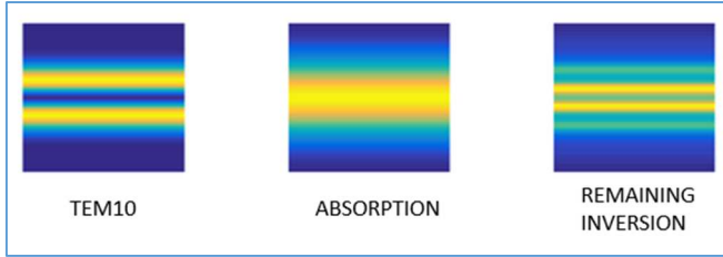
Fig 2. Plot of TEM 10 mode, initial carrier density inside the active region and remaining inversion after TEM 10 oscillation.
