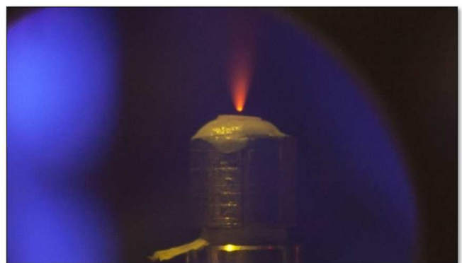
Fig. 8. Helium gas jet produced by a de Laval nozzle in vacuum, exhibiting a plasma excited by ultrashort pulses. The jet shape can be observed by the light emitted by He moving at supersonic speeds out of the laser interaction region.
