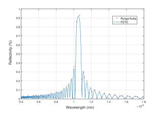
Fig. 3. Comparison between 4th-order-Runge-Kutta method and FDTD method. The red points represent the Runge-Kutta solution and the blue line represents the FDTD solution to 30 gratings.
