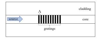
Fig. 6. Schematic diagram of fiber Bragg grating used in two-dimensional problem.
