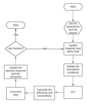
Fig. 2. Flowchart of FDTD algorithm implementation.
