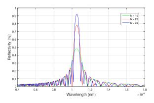
Fig. 4. Variation of the reflectivity coefficient for three different values of number of periods. It is possible to see that the greater is the gratings number, the stronger is the reflectivity.
