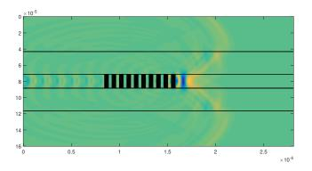
Fig. 7. Two-dimensional 1018nm FBG simulation to 10 gratings periods.
