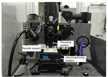
Figure 1. Initial setup for producing nanoparticles via PAL technique with femtosecond pulses.
