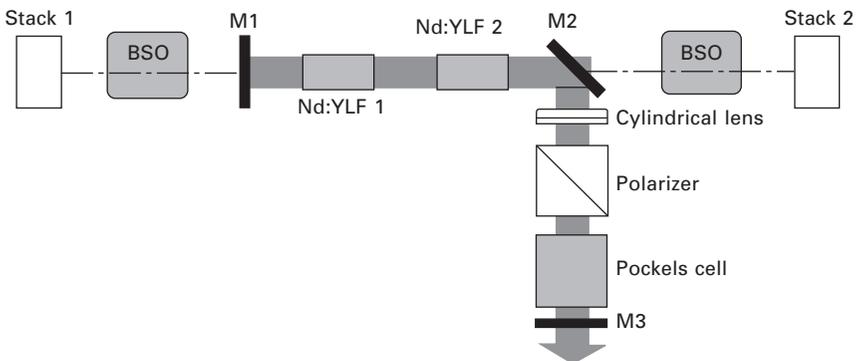
12.4 Unstable folded resonator design with diffraction-limited output employing two Nd:YLF crystals pumped by two diode stacks and beam-shaping optics (BSO) (Li *et al.*, 2008).
