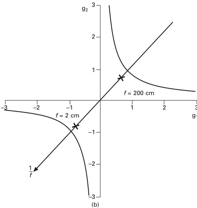
12.2 Example of joint stability zones in a side-pumped laser. (a) Simple high-efficiency resonator with equal distance between crystal and mirror M1 and M2, respectively. (b) Joined stability zones of this resonator, permitting stable operation with a thermal lens ranging from 200 cm to 2 cm as a function of pump power (Wetter *et al.*, 2008a).
