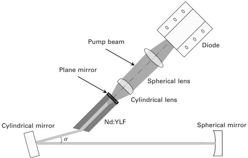
12.3 End-pumped laser cavity scheme. This folded cavity uses a cylindrical mirror in order to match laser and pump beam inside the Nd:YLF crystal (Zehetner, 1995).
