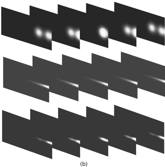
12.5 (a) Double pass through side-pumped Nd:YLF. (b) Five  $xy$ -slices of the diode-side-pumped region of the Nd:YLF crystal. Top to bottom: two  $TEM_{00}$  modes undergoing total internal reflection at the pump surface; absorbed pump power inside crystal; overlap of the two  $TEM_{00}$  modes with the pump inversion (Wetter *et al.*, 2009).
