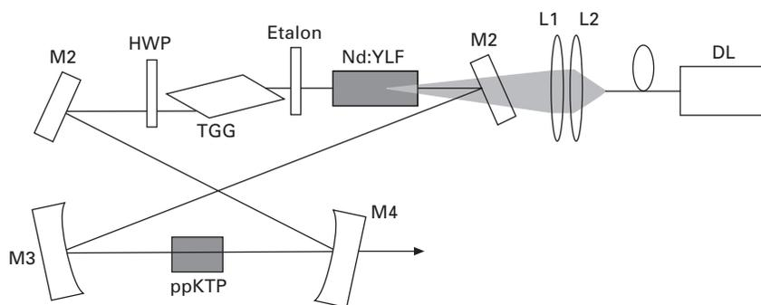
12.6 Single-frequency, tunable ring-cavity for efficient SHG conversion to the red (Camargo *et al.*, 2009). M1–M4 are the ring-cavity mirrors, HWP is the half-wave-plate that together with the TGG makes the optical diode, L1 and L2 are the two doublet lenses that focus the fiber-coupled diode laser (DL) into the Nd:YLF crystal.
