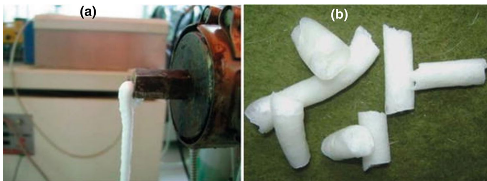
Fig. 4 Structural foams: a extruded foams from a 4 mm die extruder; b cylinder structural foams, of approximately 400 \text{ kg}\cdot\text{m}^{-3} density (Reprinted with permission from IntechOpen) [68]
