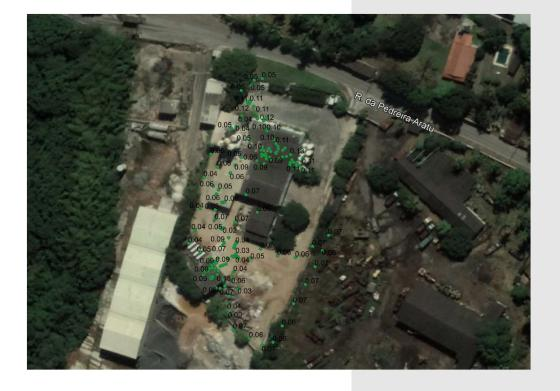
The radiometric survey of the working area was evaluated by using a Geiger-Muller. The mean exposition rate was  $0.07 \mu$ Sv/h (0.6 mSv/y).
