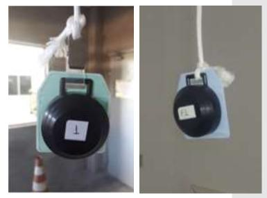
Dosimeters CR-39 and TLD installation before and after the application of the mortar
