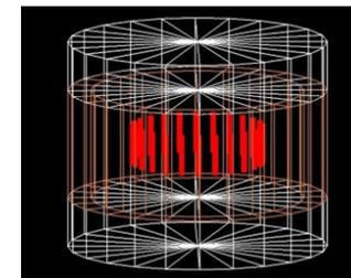
Figure 1: GammaCell 220 simulated geometry from TOPAS code.
