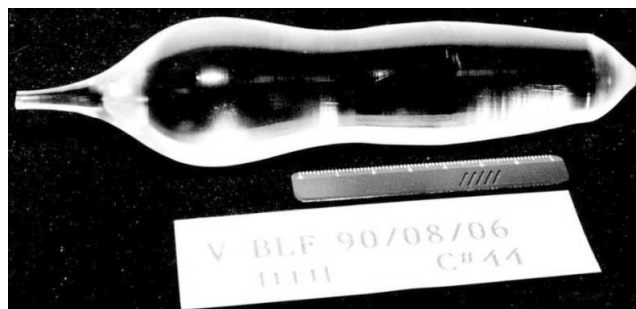
Fig. 5. Large BLF crystals growth by CZ method under Ar and \text{CF}_4 atmosphere.
