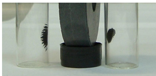
Fig. 4 Magnetic responses of the MAG (left) and MZ (right) in contact with a magnet
