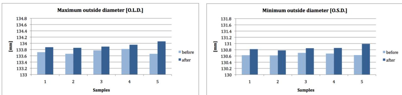
Fig. 7. Differences of maximum and minimum outside diameter before and after laser process for five different ring samples.
