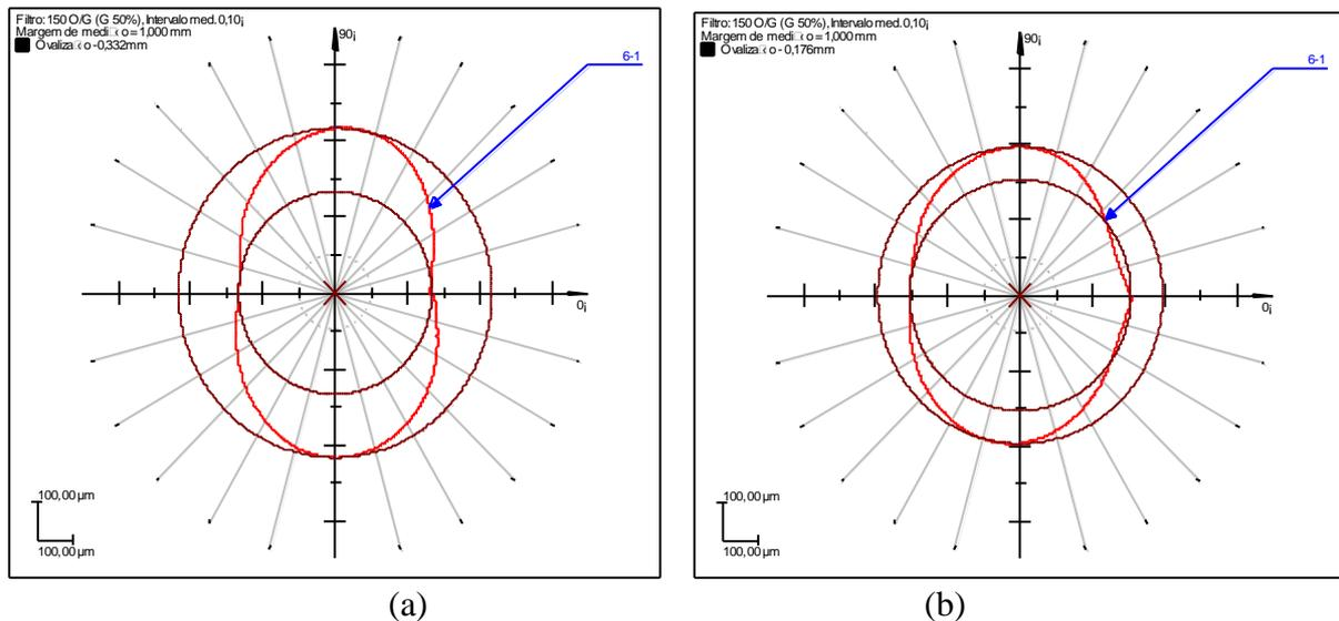
Fig. 9. a) Ovality graph for the ring before laser processing. b) Ovality graph of the ring after laser processing.
