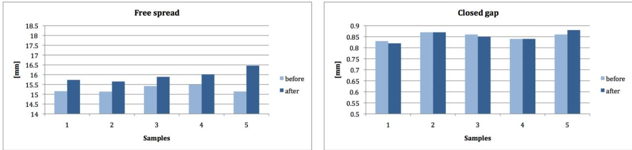
Fig. 8. Differences of free spread and closed gap parameters before and after laser process for 5 different ring samples.
