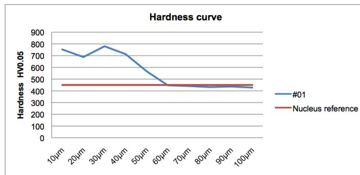
Fig. 6. Case depth average Vickers hardness values, under influence of laser irradiation process, measured for the peripheral surface of the ring.
