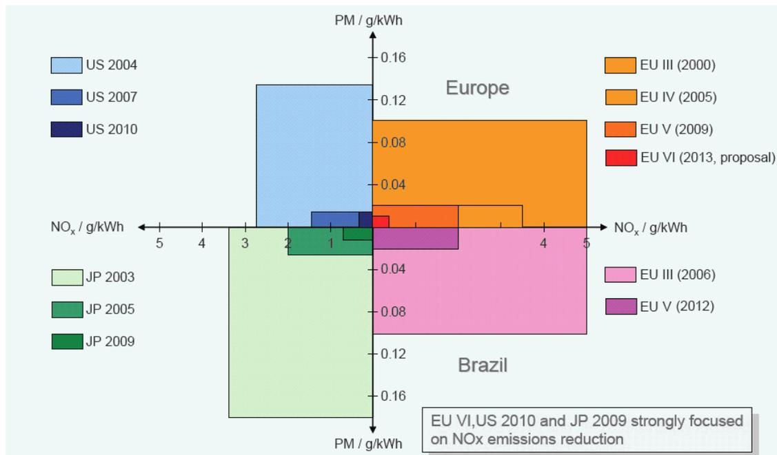
Fig. 1. Emission legislation map for HDD engines [2].
