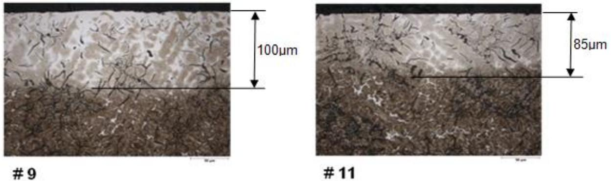
Fig. 4. Optical micrograph showing detail of samples #9 and #11 of ring section under influence of chosen irradiation parameter as showed in Table 1. Nital 3% etch.
