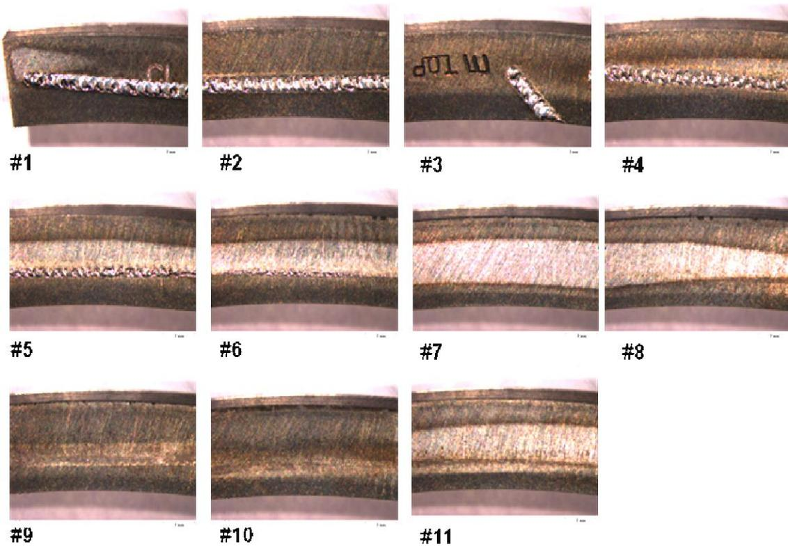
Fig. 2. View of lateral surface of the piston rings under influence of different laser irradiation parameters.
