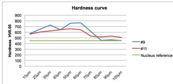
Fig. 5. Case depth average values hardness considering samples #9 and #11, under influence of different irradiation parameters.
