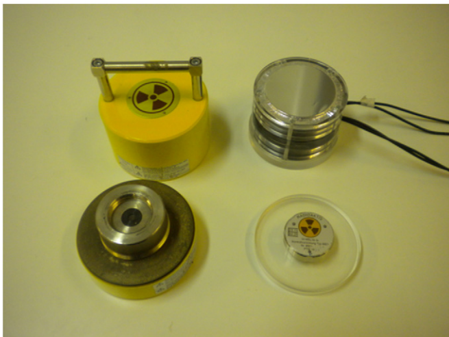
Fig. 1. Double faced ionization chamber and the check source positioned on the support apparatus.
